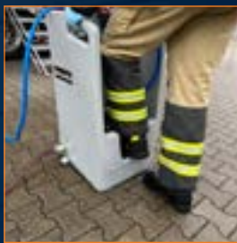
BOOT WASHING MACHINE Cleaning boots and equipment
