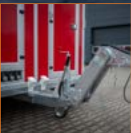
HEIGHT-ADJUSTABLE DRAWBAR Tool-free and vehicle-independent
