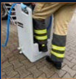
BOOT WASHING MACHINE Cleaning of boots and equipment
