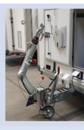
Height-adjustable drawbar with exchange coupling
