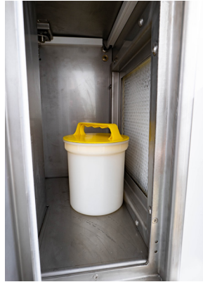
Safe sample transfer via negative pressure airlock
