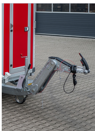
Height-adjustable drawbar with exchange coupling
