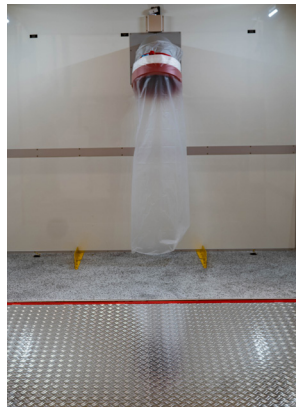
PPE disposal ends in a continuous liner bag
