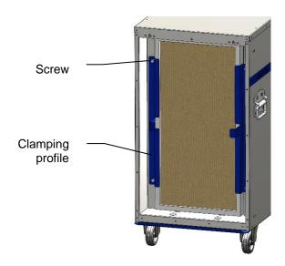
Remove clamping profiles
