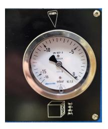
The following table shows the display values for a recommended filter change. If the display reaches this value, please replace the pre-filter first. If the display value drops by 100 Pascal or more, the appliance can continue to be operated. If the value drops by less than 100 Pascal, the HEPA filter must be replaced.
