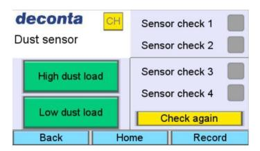
The measured values of the filter sensors can be displayed graphically using the "Record" button.
