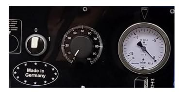
The following table shows the display values for a recommended filter change. If the display reaches this value, please replace the pre-filter first. If the display value drops by 100 Pascal or more, the appliance can continue to be operated. If the value drops by less than 100 Pascal, the HEPA filter must be replaced.
