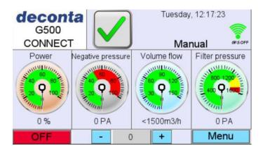
To monitor the filter, the filter pressure is shown on the control unit display. If the display reaches the red area, please replace the pre-filter first. If the display value drops by 100 Pascal or more, the appliance can continue to be operated. If the value drops by less than 100 Pascal, the HEPA filter must be replaced.
