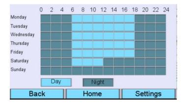
By selecting time ranges, you can set here on which days and at what time the value set in automatic mode for the minimum negative pressure in night mode (min. negative pressure night) is activated.
