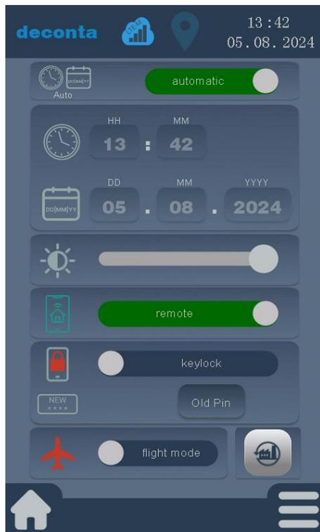
Tapping on the "Old Pin" button opens a window with a request for the previous pin.
