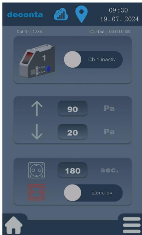
An additional Negative pressure unit can be connected to the alarm socket of the aircontrol connect in standby mode. This is switched on when the negative pressure falls below the set value for low alarm and the delay time has elapsed.
