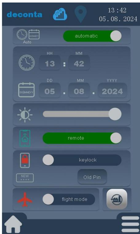
The device can be set to flight mode. This disconnects GPS, WiFi and mobile data.
