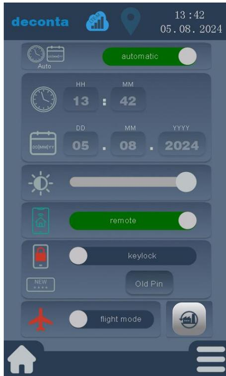
Setting the display brightness. The brightness can be changed using a slider.
