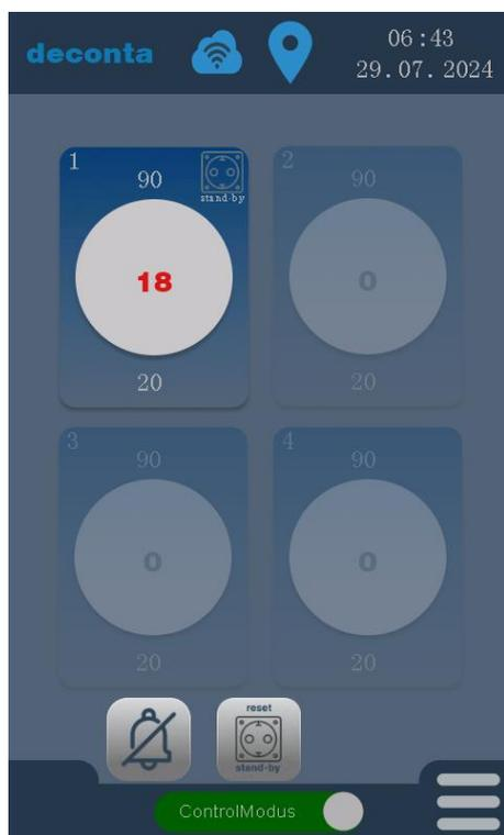
If the standby function for the socket is active in the settings of the measuring channel, the function is displayed below the socket symbol.
