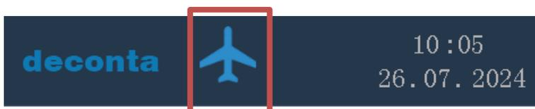
Device is in flight mode, data connections and location determination are deactivated
