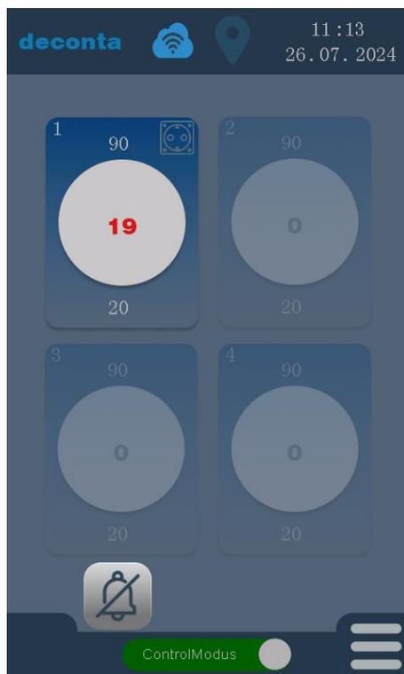
After the delay time has elapsed, the measured negative pressure is displayed in red and an alarm is triggered.
