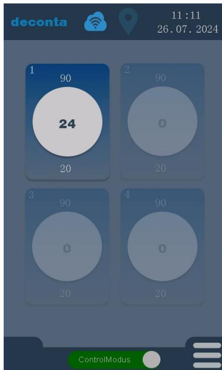
Measuring channel 1 is activated, channels 2, 3 and 4 are deactivated and are greyed out.
