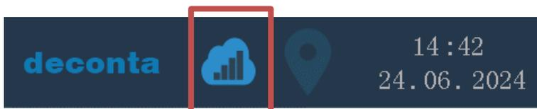
Connected to deconta decoNXT via mobile data
