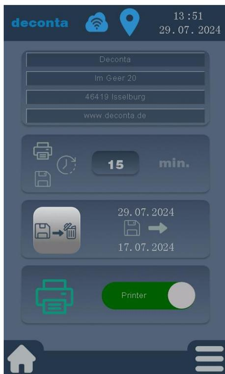
The output of measurement data via the printer can be activated or deactivated.
