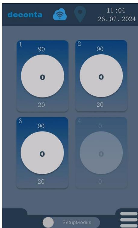
The settings of the respective measuring channel can also be called up directly by tapping the channel on the main page.
