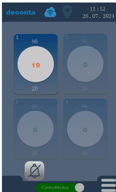
The measured negative pressure (19 Pa) falls below the set value (20 Pa) for the alarm low, the adjustable delay time starts to run.
