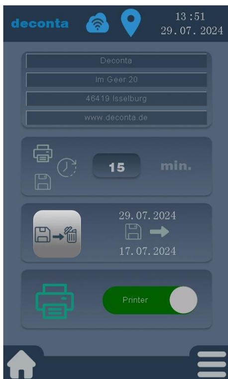
A customer-specific text (e.g. an address) can be entered here in 4 lines, which is then printed on the printer.
