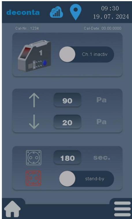
The high and low alarm values are set by tapping the number field next to the up or down arrow.
