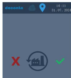
After resetting, the device restarts with factory settings.
