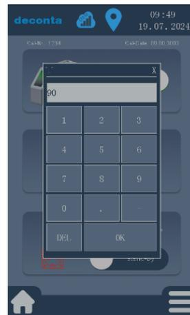
The delay time for activating the alarm socket is set by tapping on the number field next to the socket symbol.
