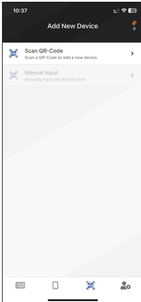
As an alternative to scanning the QR code, the key displayed on the aircontrol above the QR code can also be entered by tapping on "Manual Input".
