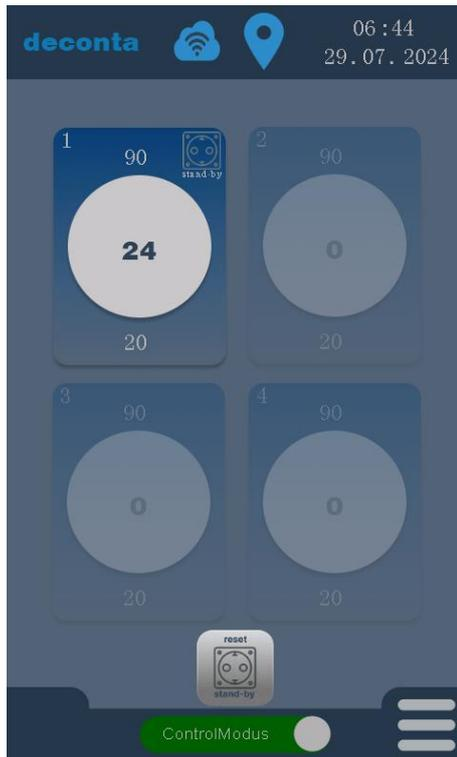
When the measured negative pressure is back within the limit values, the socket for the connected standby device can be switched off again by tapping the "reset standby" button.
