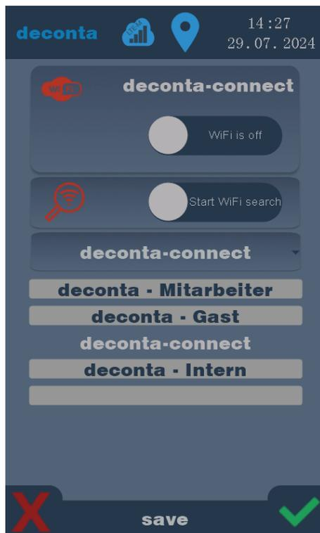
The available networks are displayed. Select the desired network and confirm by tapping the green tick.
