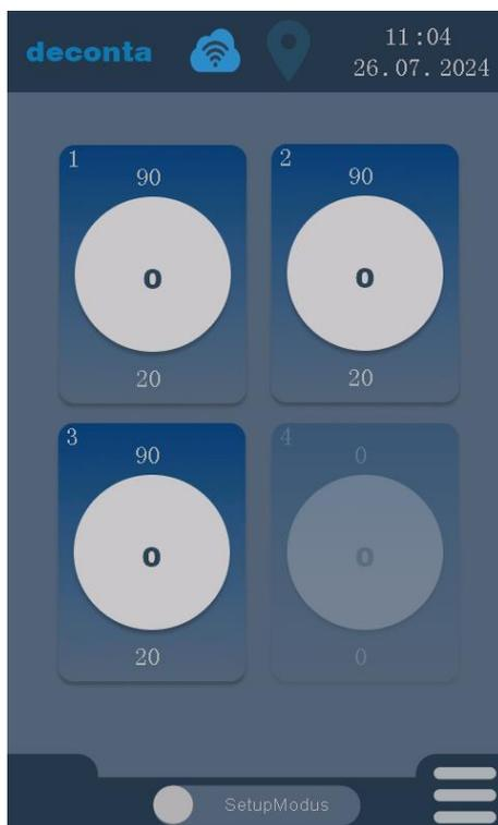
Once all parameters have been set, the negative pressure measurement can be started by tapping the "Setup mode" button.
