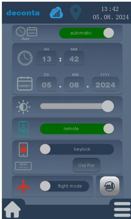
A key lock can be switched on or off using the "keylock" button.
