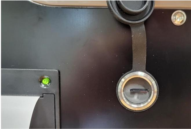
The slot for the memory card is located on the side of the device behind a protective cap. If no memory card is inserted, the message "SD missing" is displayed on the main page.
