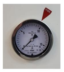
The value for a recommended filter change is marked with a red arrow.
