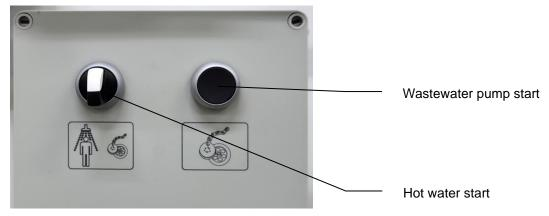
The wastewater pump can be switched on manually by pressing and holding the "Wastewater pump start" switch.
