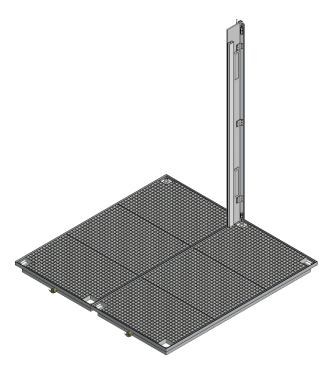
Insert a corner profile with pre-assembled roller shutter guide at the connecting corner of two floor units in the mounting brackets and tighten the quick-release fasteners attached to the ends of the corner profiles with the floor units.
