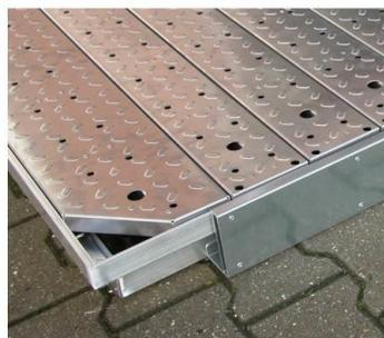
Insert a corner profile at the connecting corner of two floor elements into the mounting brackets and tighten the quick-release fasteners attached to the ends of the corner profiles to the floor elements.
