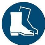
Risk of crushing: Wear safety shoes to protect limbs from being run over.
