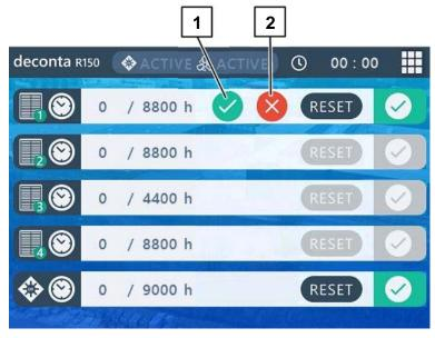
Abb. 16 RESET button for resetting the operating time
