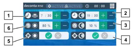
Abb. 10 Interface for setting the operating parameters
