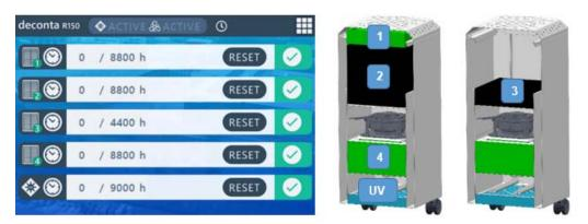
Abb. 14 Operating hours and recommended operating time of the individual stages
