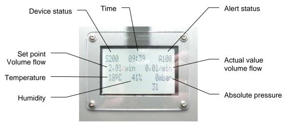
After switching-on the device, 3 pieces of information appear on the upper line of the display:
