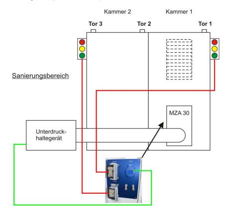
Connect the measuring hose to the control unit (connection) as shown in the following picture and place it in the sanitation area.
