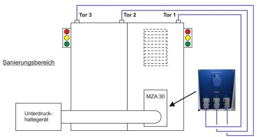
Connect the traffic light system to the control unit MZA 30 as shown in the following picture (labeled with traffic light).
