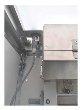
Connect the supplied electrical cables to the three connections on the outside of the roof (where the plugs are also connected from the inside) and connect the control compulsory locking. It does not matter in which order the three plugs are connected to the controller.
