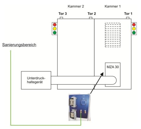
Connect the power supply to the lock control unit MZA 30.
