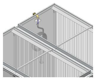
Place the connecting profile where two floor elements are adjacent to each other. This prevents water from escaping from the airlock.
