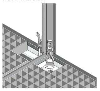
Insert the wall element into the mounting brackets of the floor element and the corner profile.
