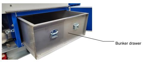
• The bunker drawer can now be pulled out and the contents disposed of according to regulations.
