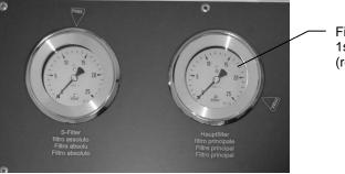
Filter monitoring 1st filter stage (regenerative filters)
