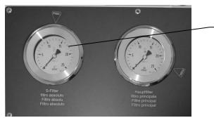
Filter monitoring 2nd filter stage (HEPA filter)
