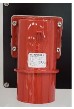
The dust extractor is equipped with a 32 A surface-mounted appliance plug. It is connected to the electrical power supply with a CEE plug.
