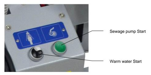
By pushing and holding of the button "Waste water pump Start" the Waste water pump can be switched on manually.
